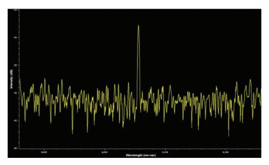
100 Hz Pulse Rate 5,000 pulses collected OSNR ~ 10 dB Measurement Time ~ 100 seconds
