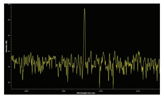
**100 Hz Pulse Rate** 30,000 pulses collected OSNR ~ 16 dB Measurement Time ~ 10 minutes
