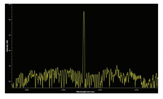
10 kHz Pulse Rate 100,000 pulses collected OSNR ~ 20 dB Measurement Time ~ 20 seconds
