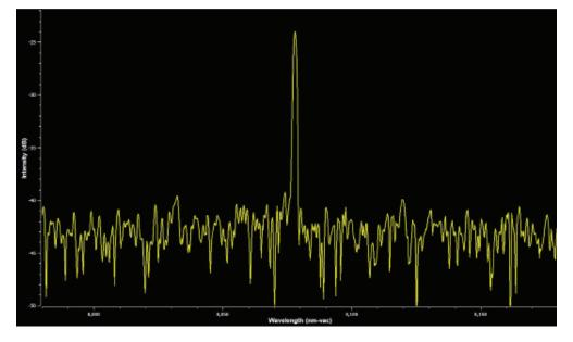
30 kHz Pulse Rate 100,000 pulses collected OSNR ~ 20 dB Measurement Time ~ 10 seconds
