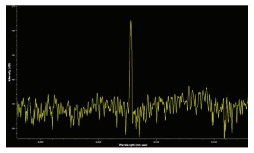
**5 kHz Pulse Rate** 30,000 pulses collected OSNR ~ 16 dB Measurement Time ~ 12 seconds
