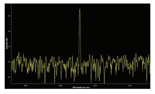
1 kHz Pulse Rate 30,000 pulses collected OSNR ~ 16 dB Measurement Time ~ 60 seconds
