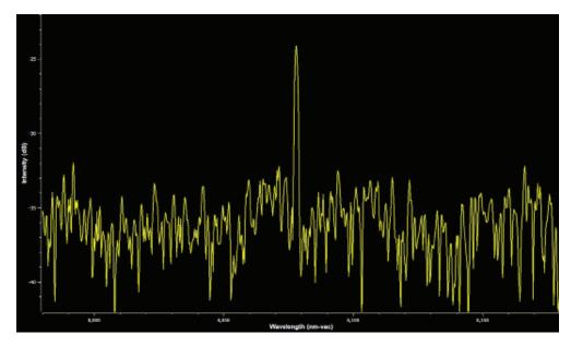
1 kHz Pulse Rate 5,000 pulses collected OSNR ~ 10 dB Measurement Time ~ 10 seconds
