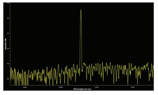
**5 kHz Pulse Rate** 100,000 pulses collected OSNR ~ 20 dB Measurement Time ~ 40 seconds
