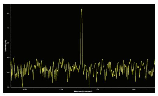
100 kHz Pulse Rate 100,000 pulses collected OSNR ~ 20 dB Measurement Time ~ 10 seconds
