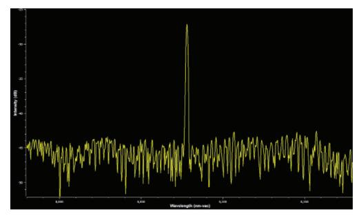
10 kHz Pulse Rate 30,000 pulses collected OSNR ~ 16 dB Measurement Time ~ 10 seconds
