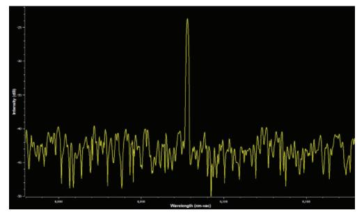
**50 kHz Pulse Rate** 100,000 pulses collected OSNR ~ 20 dB Measurement Time ~ 10 seconds
