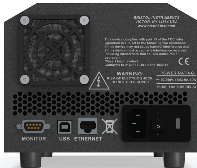
Figure 22. 771 system rear panel connection layout.
