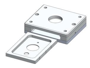
This Group Index Cell consists of a fixture that holds a pair of air-spaced flat optical plates and a sliding tray that is used to hold a material sample and position it between the two optical plates. The sample must be able to fit in the cell and can consist of only one material.
