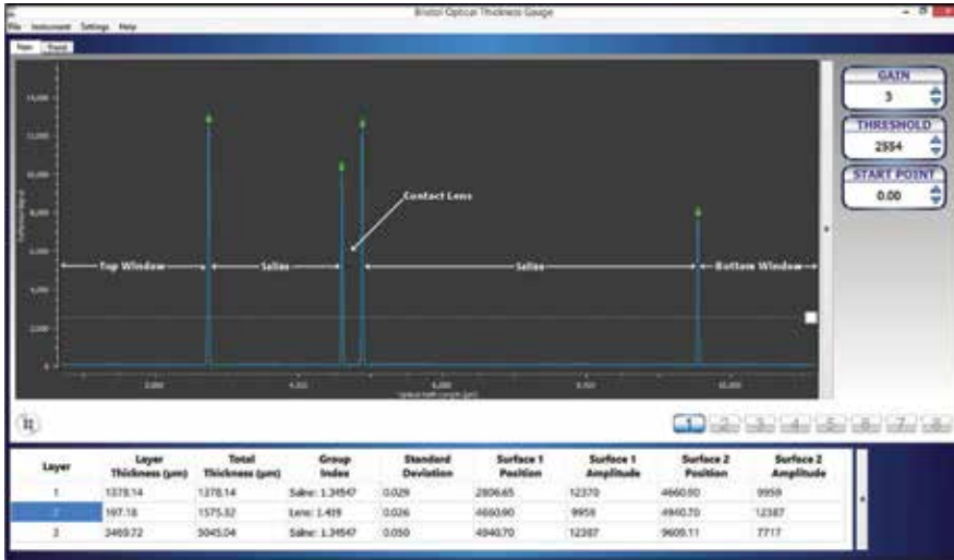
Figure 4. An example of a measurement of a soft contact lens immersed in saline solution.
